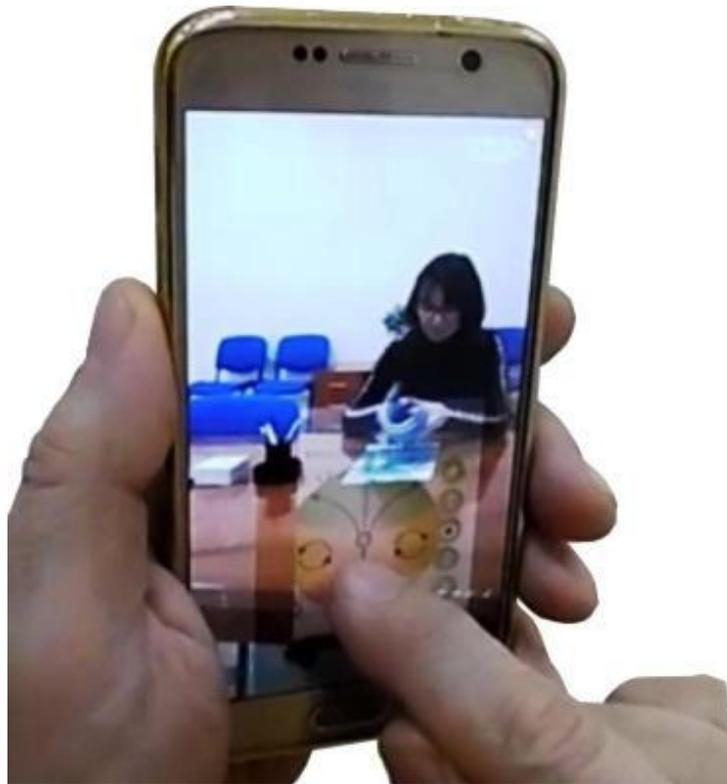
Fig. 3. Robot controlling disk opened in foreground of Skype in floating browser
